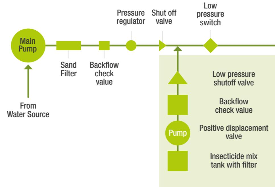
**Basic drip irrigation system using a positive displacement injection metering pump:**
