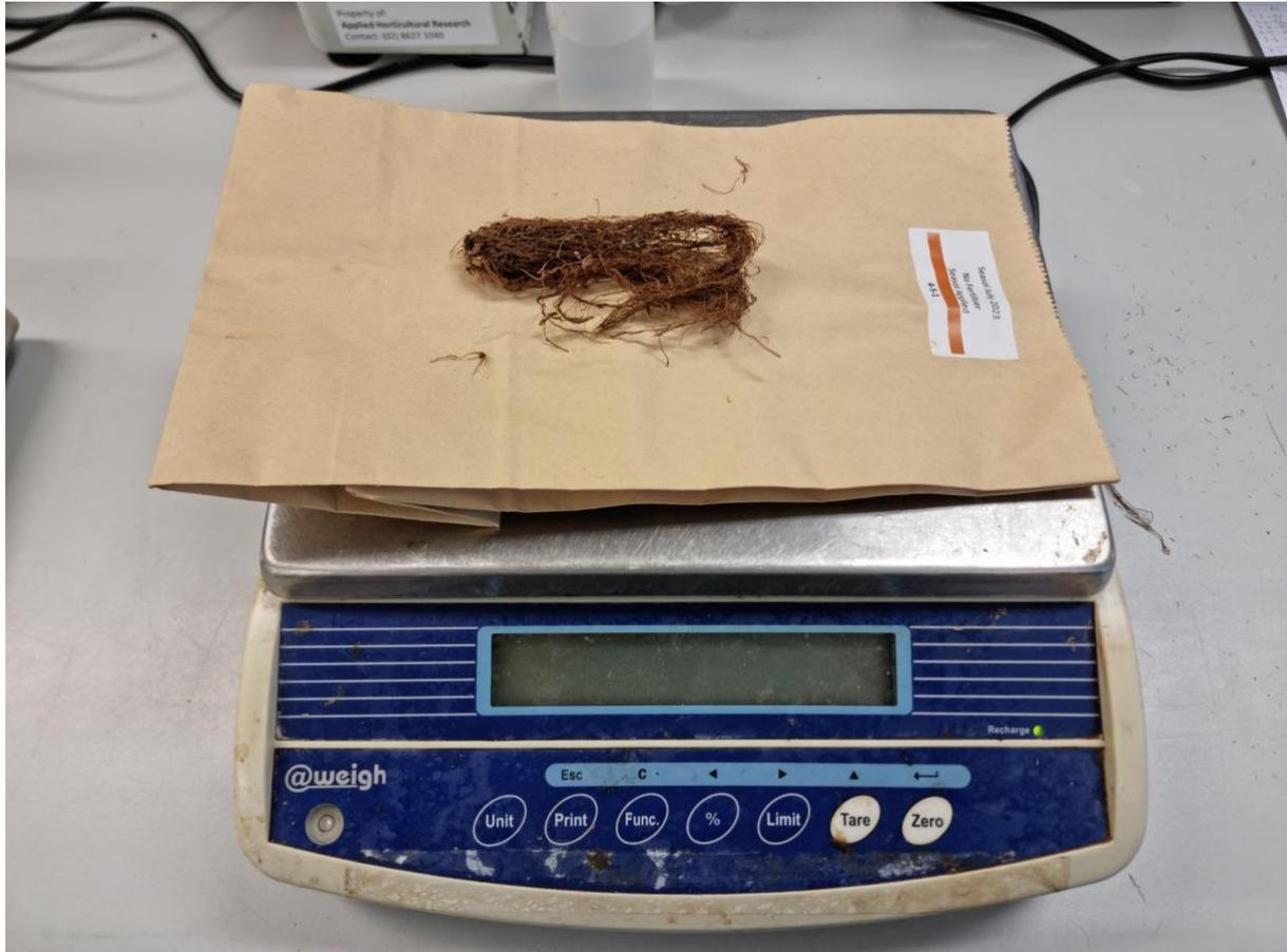
**Figure 22:** Roots were weighed after drying.
